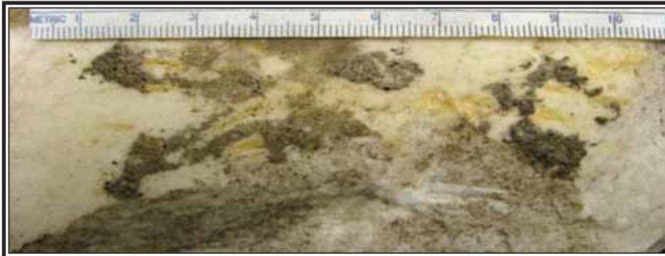
Figure 5: A closer view of the mortar remnants present on the flat back side of the "Isis" white marble artifact.
